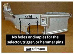
ATF's definition of a receiver excludes those it deems "less than eighty percent" complete. See its graphic (we enlarged some of the text for clarity). As much an object might *look* like a receiver, if it lacks "holes or dimples for the selector, trigger or hammer pins" it's "Not a firearm." Problem is, kits are widely available that furnish all the parts, templates and instructions for making functioning, non-serialized "ghost guns" in one's workshop, or at home. DOJ's
